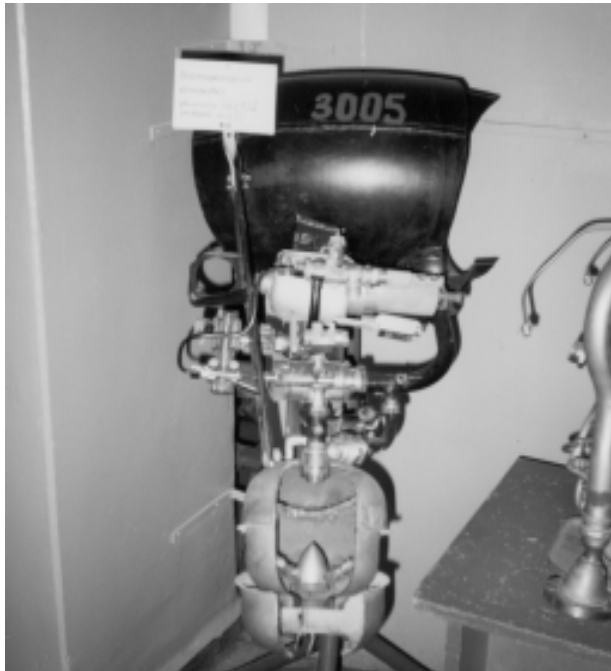
Fig. 10 The RD-101 steam generator with its solid catalyst - a cutaway demonstration model.
