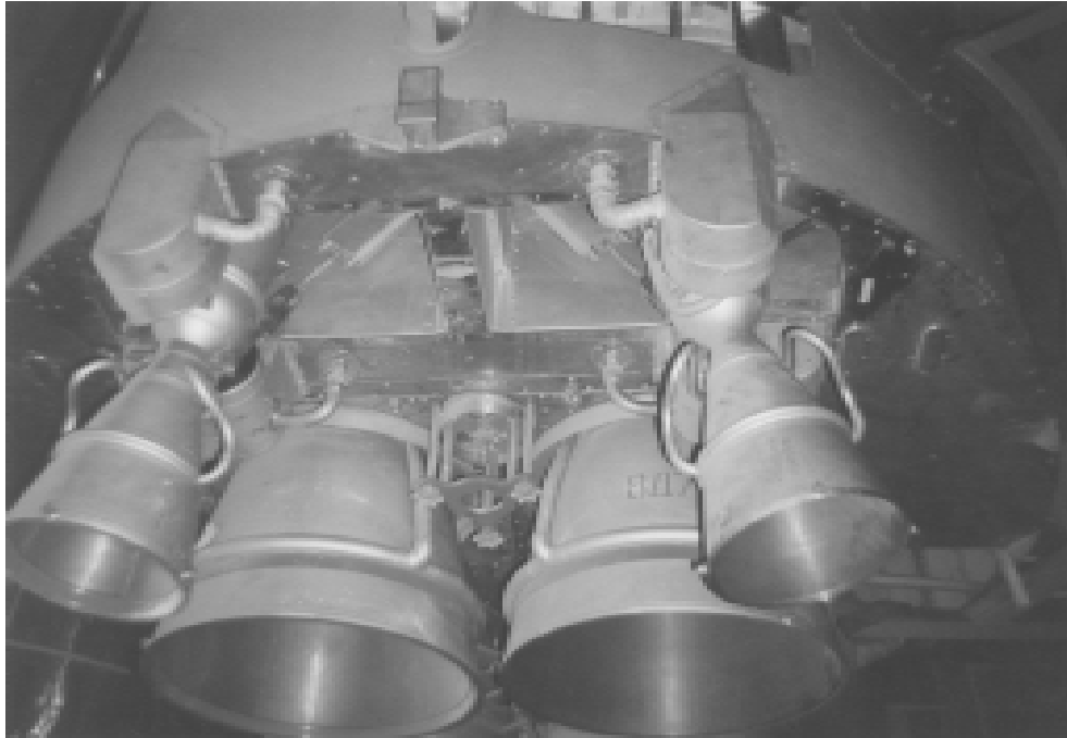
Fig. 36 The RD-107 as built in the first stage of the R-7.
